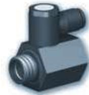
The piloted vacuum valve CSP series mounts directly on the suction cup and allows to maintain the vacuum in it, in case of emergency stop or malfunctioning of the vacuum generator.
