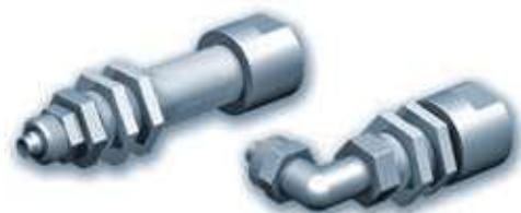
The L series extensions are used for gripping on various levels using the same installation plate. These extensions are adjustable to different heights. This system is especially useful for 2.5 bellows type suction cups, as height adjustment is made easier by the deflection of the suction cup. Spring systems should be chosen, instead, for flat suction cups with low deflection.
