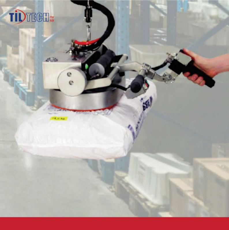
With Lifts All's sack gripper you can lift all types of bags quickly, safely and ergonomically.
