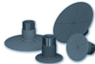
Developed through partnerships with the composite material industry, the VPSC suction cups are dedicated to the handling of raw composite. Their ultra-flat profile and innovative system of vacuum distribution across the surface of the cups provide optimized gripping with no mark and no deformation. The extra thin sealing lip contours to the product shape without restriction.
